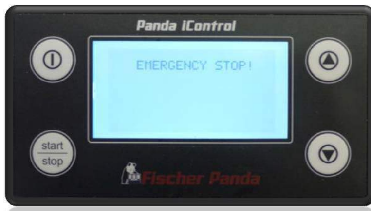
Fig. 12.5-2: Panel shows Emergency Stop
