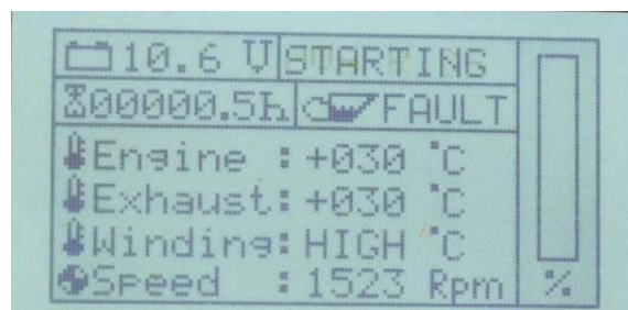
Fig. 16.1.1-2: Warning: „Winding temperature too high“
