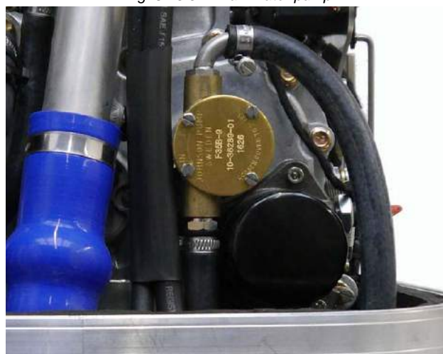
Fig. 8.13.3-2: Raw water pump
