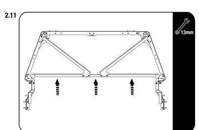
Using clamps and a spirit level clamp the spirit level to the inside of the Front Center Brace and Tighten the M6x20 Button head screws and M6 Nyloc Nuts fitted in 2.3.
