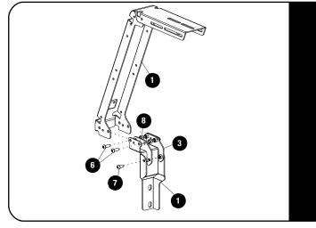
Assemble the Pro Bed Leg (Item 1) on page 3 and the Front Mounting Bracket (Item 1) to using M8 x 20 Button head bolts and M8 nyloc nuts (Item 6 & 8) as shown and M8 x 16 Button head bolts and M8 nyloc nuts (Item 7 & 8).
