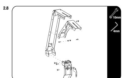
Fit the Rear Brace (Item 2) using the M6x12 button head screws and M6 Nyloc nuts (Item 14 & 8).
