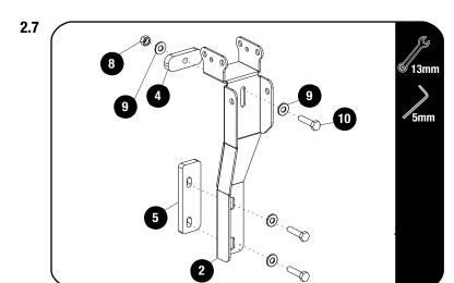
Loosly assemble the Rear Mount Brackets (item 2) using the M8x35 Hex Bolt and M8 x 19 x 2 flat washer (Item 9 & 10) in the bottom two holes in the bracket.DO NOT TIGHTEN.
