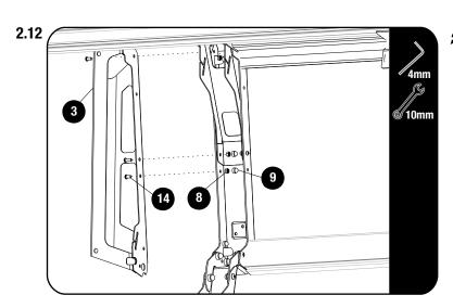
Assemble the Rear Wing Brackets (Item 3) using the M6x12 Button head screws and M6 Nyloc Nuts (Item 14 & 8).
