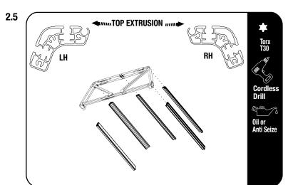
Slide the front leg and truss assembly backward to allow access for securing the extrusions.
