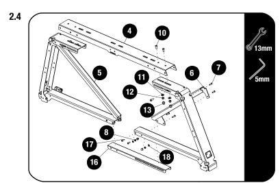
Assemble the Front diagonal and Horizontal Brace parts as shown (Item 4, 5 & 6) to the legs fitted in 2.2 using the M8 x 20 Button head bolts M8 x 19 x 2 flat washer and M8 nyloc nuts (Item 10, 11 & 12).
