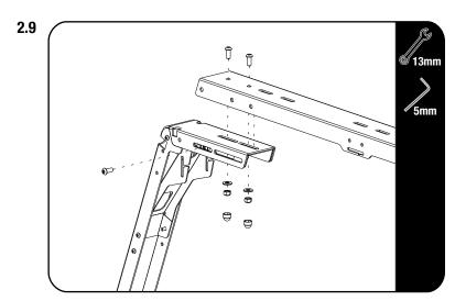
Loosely assemble the rear top truss using the M8x20 Button head screws, M8x19x2 Flat washer and M8 Nyloc Nuts (Item 10,11&12).Fully tighten the M8 Button Heads and place M8 Nut Caps on the M8 Nyloc Nuts (Item 13).
