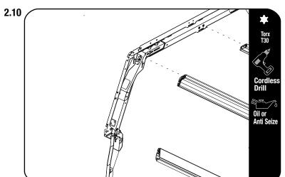
Pull the front leg / truss / extrusion assembly toward the rear legs. Attach the rear leg assembly to the Extrusions using the M6x25 thread forming screws (Item 19) and a cordless driver.The front assembly will be pulled back into its final position while fully tightening these screws.
