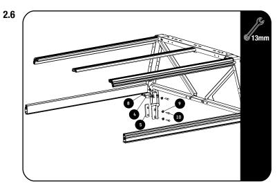
With the help of a friend lift the Pro bed rack on to the load bin and loosely fit the M8 x 35 and M8 x 19 x 2 Flat washer into the OEM mounting points together with the 10mm large spacer (Item 5,9 & 10).DO NOT FULLY TIGHTEN.
