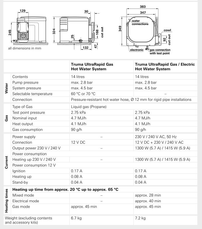
The electric heating element in the water heater is supplied with a mains cable and fitted 3-pole, earthed plug (in compliance with the norm AS/NZS 3112/2000). All other technical parameters remain the same.
