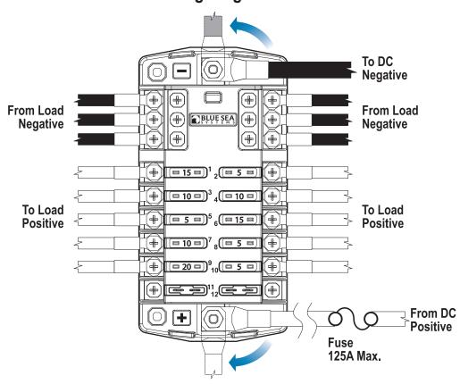
Application Note: This device is intended for branch circuit protection. Suitable main circuit protection of not more than 125A rating should be provided ahead of this device with an interrupt current rating consistent with the battery capacity.
